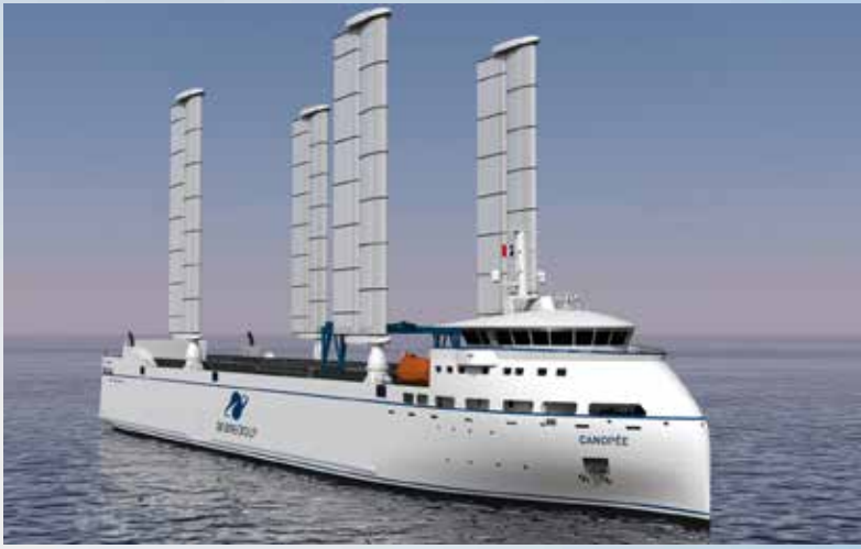
The M/V CANOPEE utilizes both wind and fuel for propulsion.
